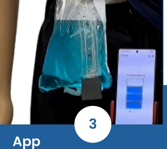
Our app offers customizable settings, allowing users to adjust bag type, volume and fill level thresholds.
